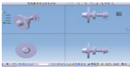
FIGURE 6 AXLE SHAFT DESIGNED IN CATIA
